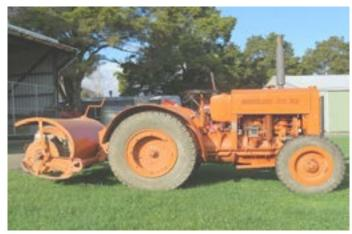
Launched in 1930, the DH22 became the first large scale production of tractors in Australia and it remained Howard's tractor line-leader for 30 years. In 1937 it was upgraded to become a 4-wheel drive. It is powered with a 22HP Morris Commercial overhead valve engine, reportedly the first overhead valve engine manufactured in Australia.
