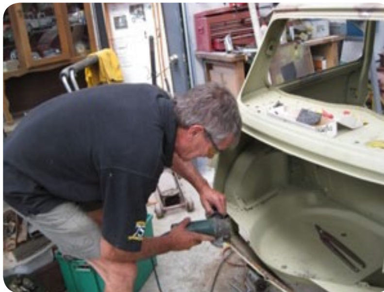
Nick Harrison cutting out rust from the trunk of the BMG Mini for Nelson Cancer
